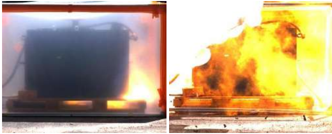
Fig. 7 Flame transmission in terminal box test
