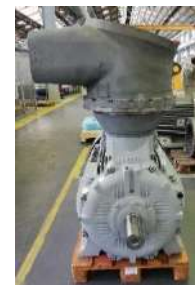
Fig. 11 – Motor subjected to modifications to comply with UL-674 and CSA 22.2 No. 145
