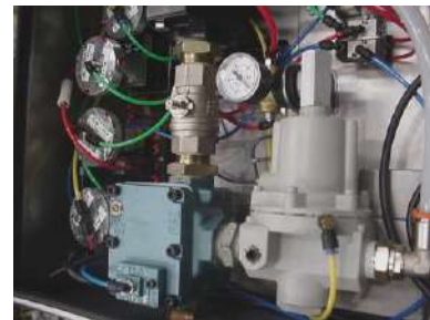
Fig. 9 Example of pressurization system installed in electric motor
