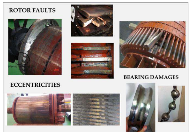
Fig. 1 Catastrophic faults in induction motors [3]
