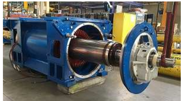
Fig. 10. Assembly of the Induction Rotor with Oil Bearings
