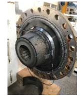
Fig. 11 Example of motor cleaning during periodic maintenance operation
