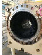
Fig. 10 Example of motor pollution by gas refouling after 5 years of operation
