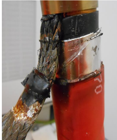
Bad connection of the earth braid because of Insulation tape forgotten
