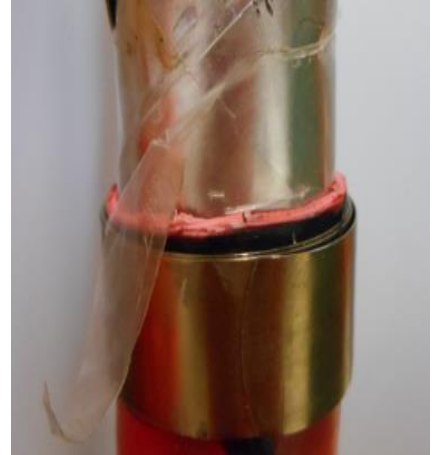
Bad connection of the earth braid because of Insulation tape forgotten
