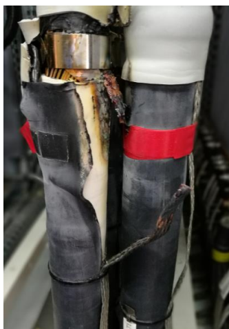
Bad connection of the earth braid because of Insulation tape forgotten
